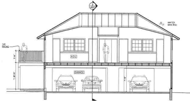
2 BUILDING SECTIONS ~ PROPOSED A3.2 1/4" = 1'-0"
