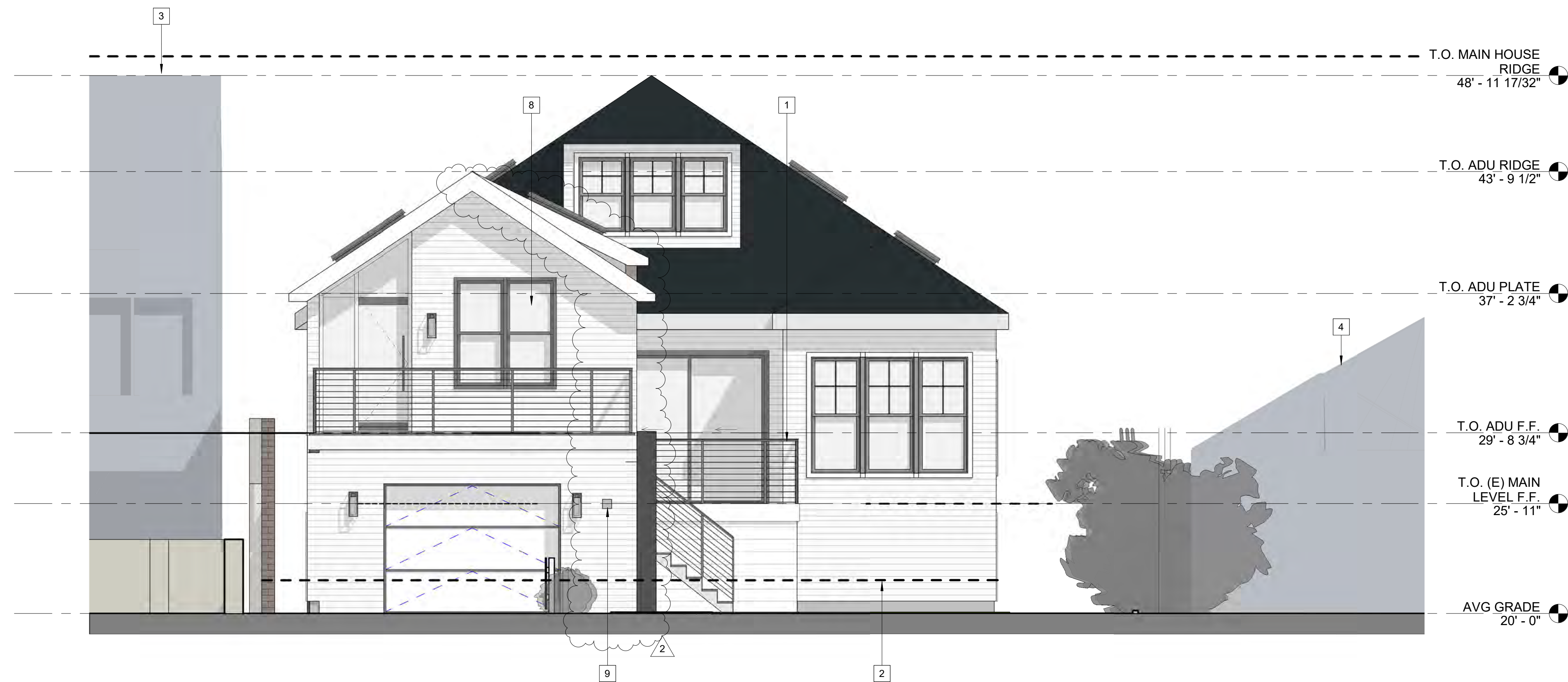
PROPOSED ADU WEST ELEVATION SCALE: 1/4" = 1'-0" 2
