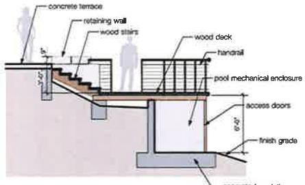
Section through proposed deck Scale: 1/4" = 1'-0"
