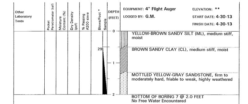
Converted to equivalent standard penetration
