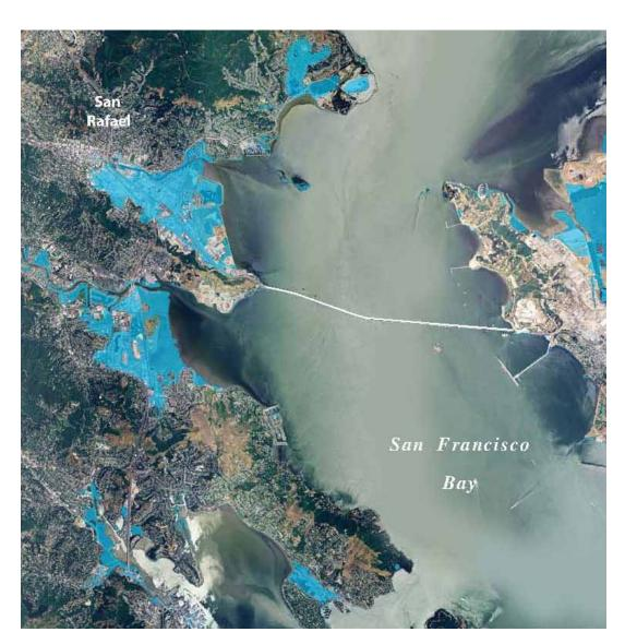
Figure 2: Inundation Effect of 16-Inch Sea Level Rise
