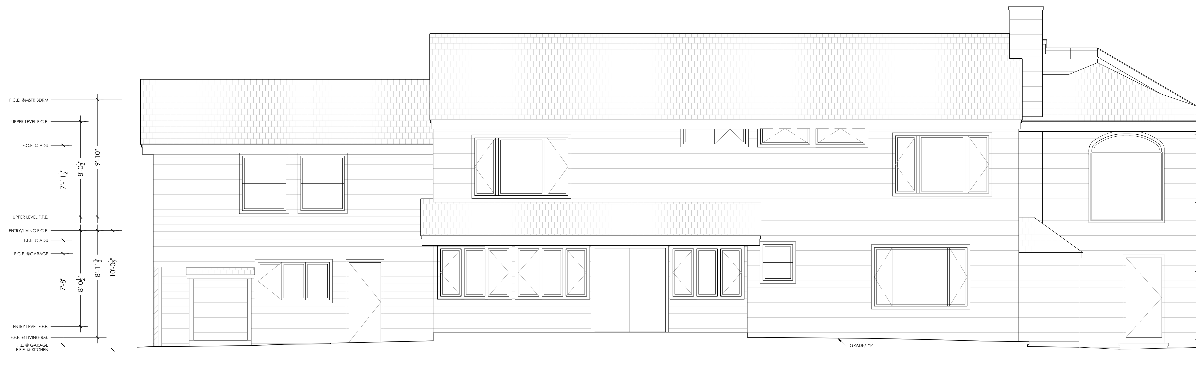
1 EXISTING NORTH (REAR) ELEVATION 1/4" = 1'-0"
