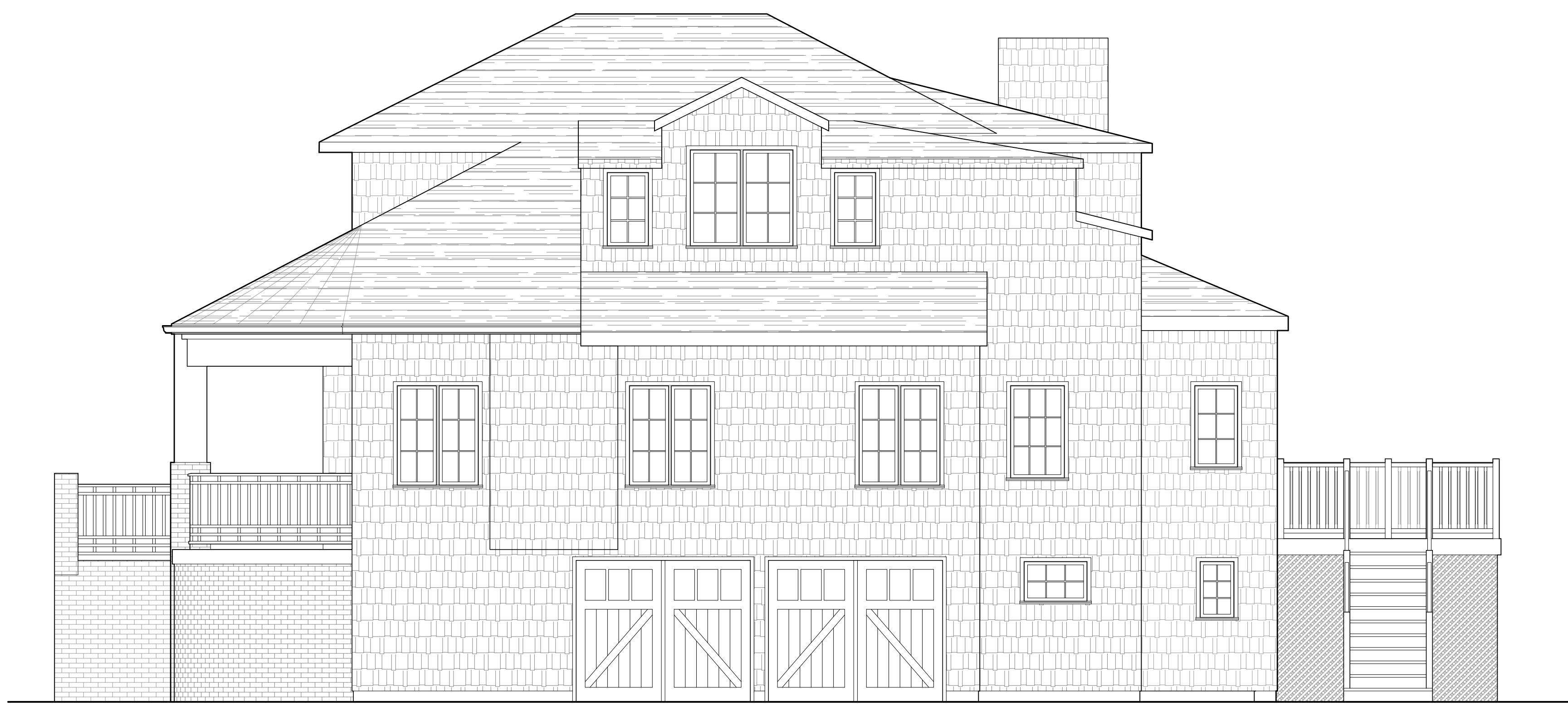
2 A3.1 EXISTING NORTH ELEVATION 1/4" = 1'-0"
